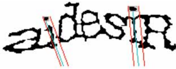
Fig. (11). The blue line is the best line to describe the line of the 'i's as calculated from the above algorithm. The area between the red lines is the estimated area of the 'i'.
