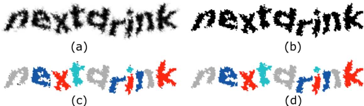
Fig. (3). Stages of Wikipedia CAPTCHA solving: (a) original character sequence, (b) thresholded, (c) connected components (d) small objects (such as noise near the n, e, t and i characters) are removed.
