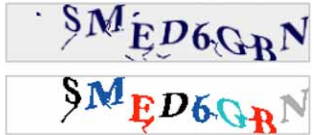
Fig. (17). Top: The initial Hotmail challenge. Bottom: Segmented character are shown in different colours.
