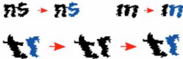
Fig. (2). Top: Examples of correct (left) and erroneous (right) Wikipedia CAPTCHA component divisions. Bottom: t and r overlap vertically and are initially combined into a single component before being split.
