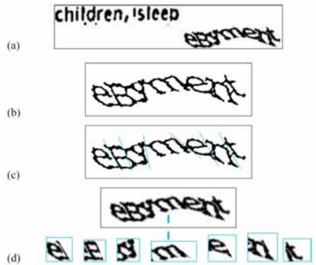
Fig. (13). Major steps in solving a reCAPTCHA challenge: (a) Initial challenge (b) The wavy word after pre-processing is done (c) The calculated segmentation lines (d) The extracted characters of the challenge
