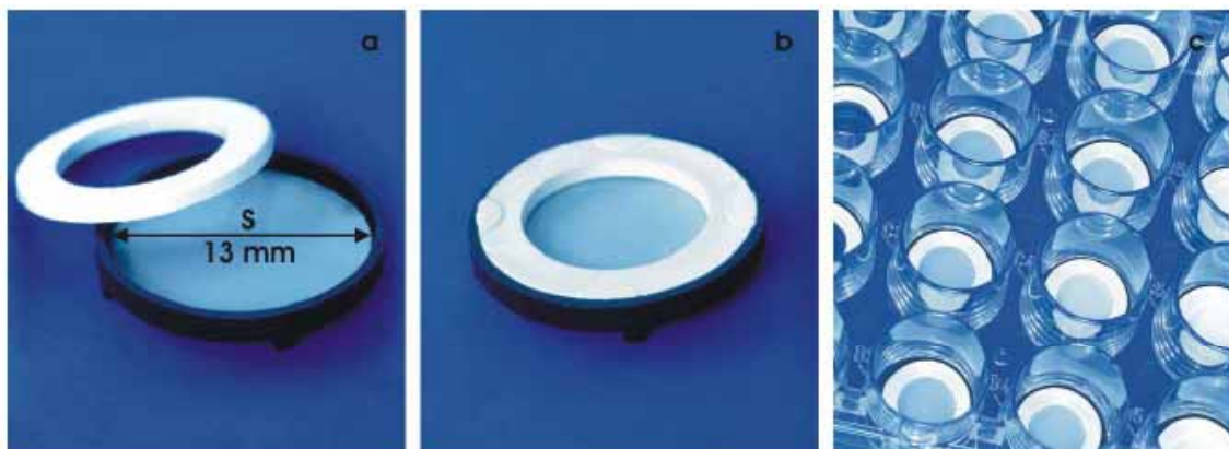
Fig. (3). Illustration of a tissue carrier used inside a gradient perfusion culture container. (a) A suitable biomaterial such as filters with 13 mm diameter is placed in a holder (black) and fixed by a tension ring (white). (b) Surface view on a mounted tissue carrier. (c) Adherence of cells is performed in a 24-well culture plate.
