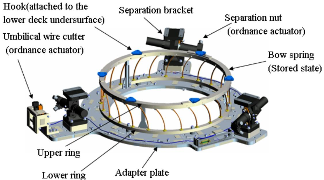
Fig. (4). Separation mechanism.
