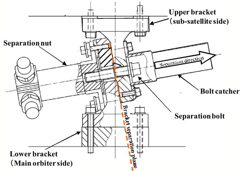
Fig. (5). Bracket mechanism.
