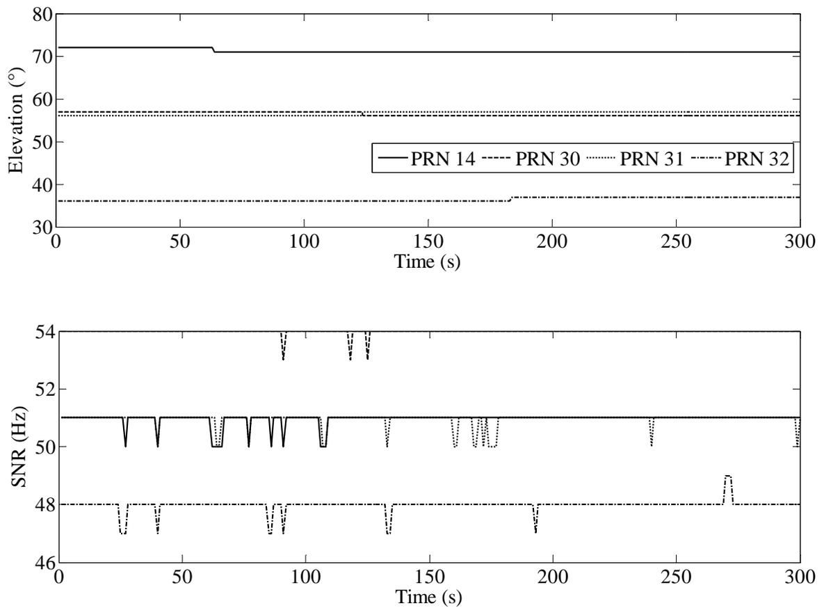
Fig. (3). Elevation angles and SNRs of satellites.
