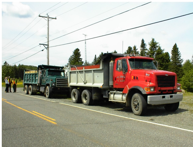
Fig. (9). Trucks used for bridge excitation.
