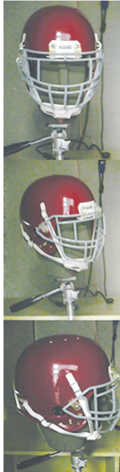
Fig. (1). Views of the dummyhead wearing the helmet as used for generation of the recordings from 0° (top), 45° (middle), and 90° (bottom), respectively.
