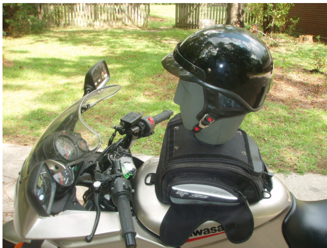
Fig. (1). Neumann KU-100 acoustically engineered dummy head with a binaural microphone system positioned at the location of the tympic membrane. The dummy head is shown with a half-helmet, the most popular style of helmet.
