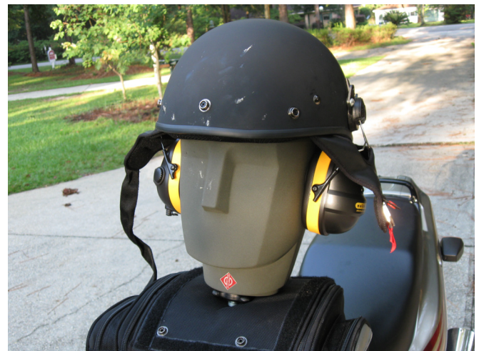
Fig. (2). Half-helmet with an ANSI certified [25 dB NPR/CSA Class A/SLC (80) 24.7 Class 4] active noise control (electronic noise cancelling) earmuff.
