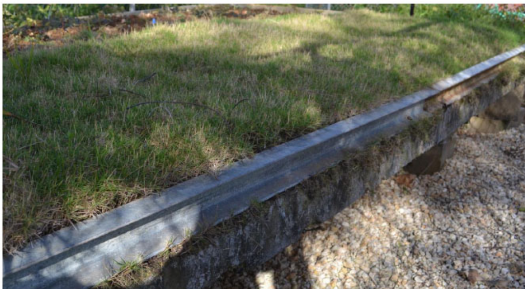
Fig. (2). Concrete plates used in the experimental structures were 0.13 m thick and resembled those used for ordinary residential roofs. Vegetation was established on half of the plates, and half were left without vegetation.
