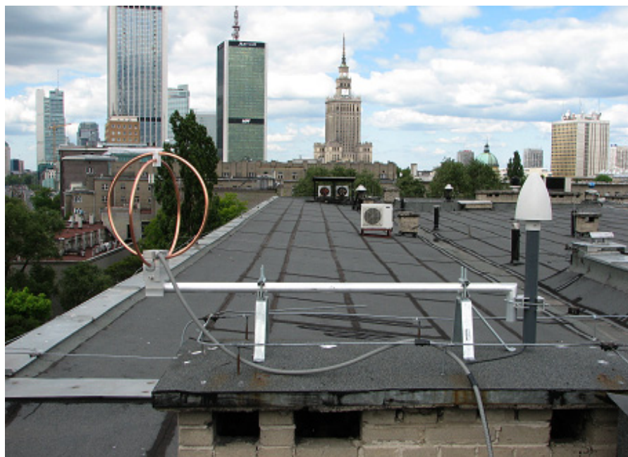
Fig. (3). View of LINET sensor set-up in Warsaw with field antenna (two crossed loops) and GPS antenna.
