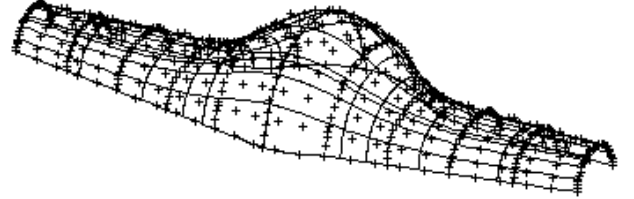
Fig. (2). The surface that interpolates the boundary curves and approximates the inner points.
