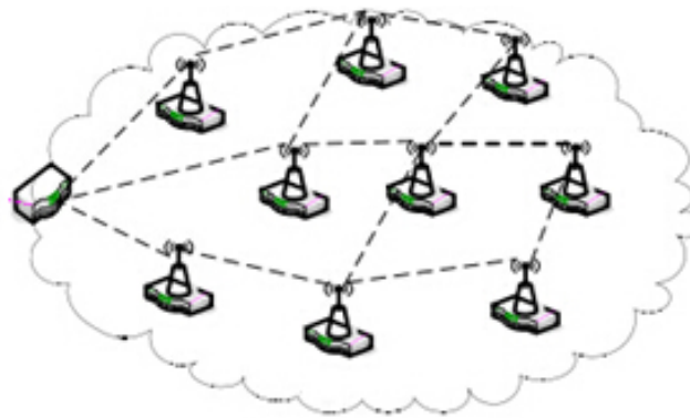
Fig. (4). Multi distributed wireless sensor network layout.
