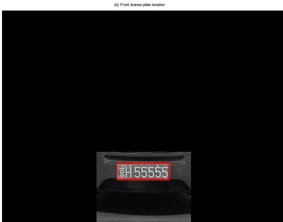
Fig. (3). The result of front license plate location of the model car.
