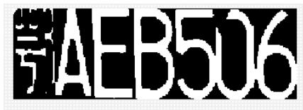
Fig. (8). Character binary images after removing the upper and lower frame.
