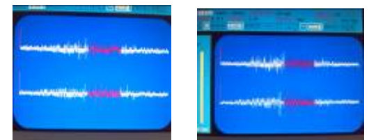
Fig. (5). Surface discharge PD pulse map under the voltage (6.3kV vs. 7.3kV).
