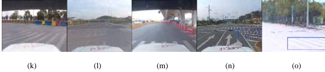
Fig.(7). Some detection results from our proposed method ( a-b: Morning; c-d: Noon; e-f: Afternoon; g-i: Partial Occluded; j-m: False Negative cause of out-of-shape、 fuzziness、 distance; n-o: False Positive cause of overlap、 reflection)
