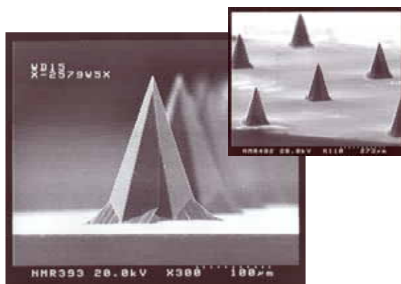
Fig. (15). Scanning electron microscope (SEM) image of solid silicon MNs.
