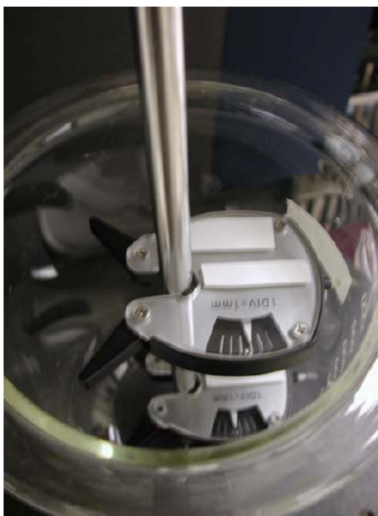
Fig. (4.2.). Vessel Centering (close-up).
