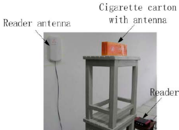
Fig. (6). Measurement setup using ALR-9800 Enterprise RFID Reader.
