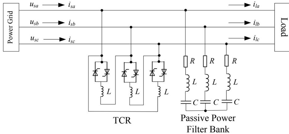
Fig. (1). Topology of TCR Compensation System.
