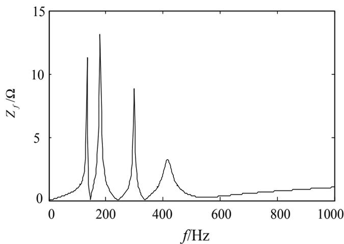
**Fig. (12).** Impedance-frequency Characteristics of PPF.
