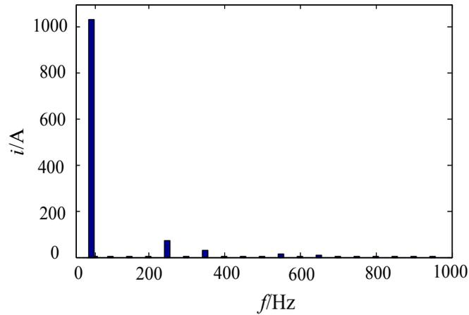
Fig. (5). Frequency Spectrum of the Current Which TCR Injecting into Phase C under Symmetrical Voltage.
