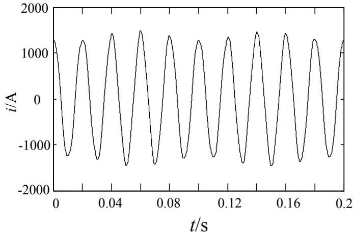
**Fig. (10).** Current Waveform of Power System after PPF Operating.
