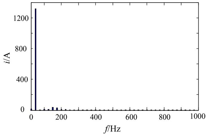
**Fig. (11).** Current Frequency Spectrum of Power System after PPF Operating.
