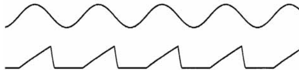
Zero-sequence voltage fifth harmonic component wave of point g and the wave of point h after positive conversion
