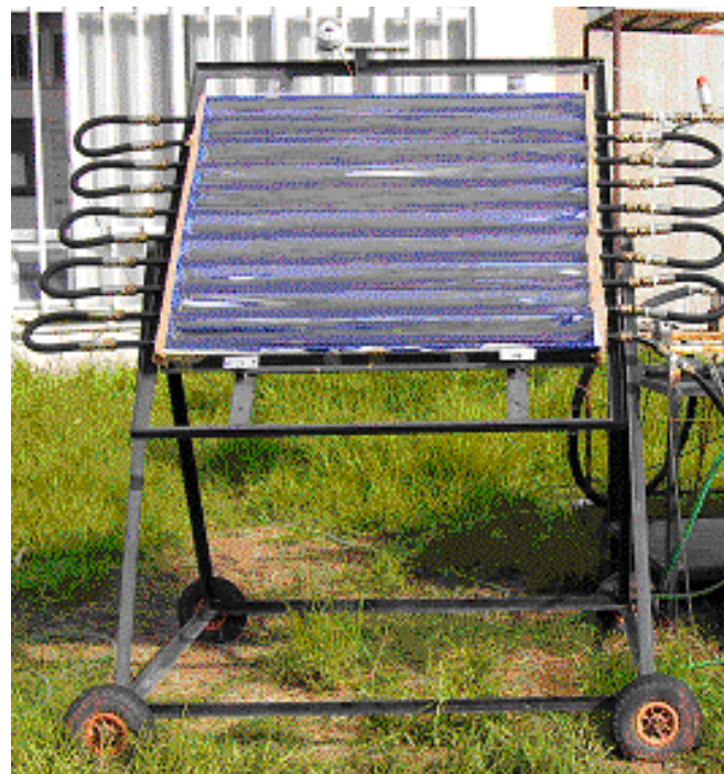
Fig. (1). A mini parabolic system of 10 reflecting parabolas connected in series constructed in the R.E.S. Laboratory.
