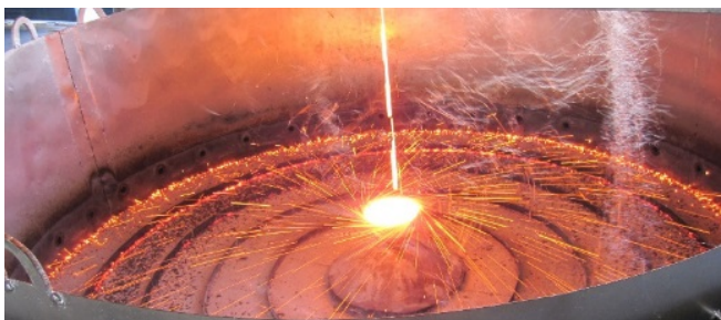
Fig. (2). Granulation process of molten blast furnace slag.
