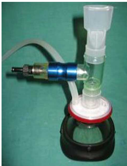
Fig. (2). Experimental ventilation device consisting of an AMBU mask size 3, a breathing filter connected to a mouth piece via a T piece. The system included a leak generated by an open Dräger ISO 15 connector size 8.0. Oxygen could be inflated via the gas detector port of the breathing filter.
