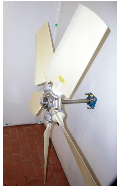
Fig. (1). Low-speed, high-volume fan used to improve air circulation in the dehydration chamber.
