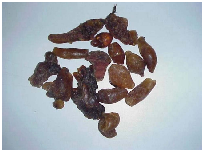
Fig. (2). Crude cashew-tree exudates samples, cleaned and free of insects or soil contamination. The resin, after being dissolved in distilled water was used for cross-linking procedures and further analysis.
