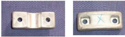
Fig. (16). Compoforged part.
