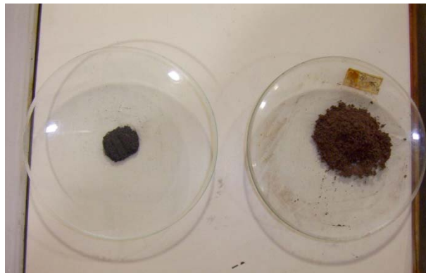
Fig. (5). \beta -SiC particles without coating (left) compared to the Cu/ \beta -SiC microcomposite (right).
