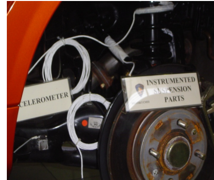
Fig. (2). Instrumented suspension system.
