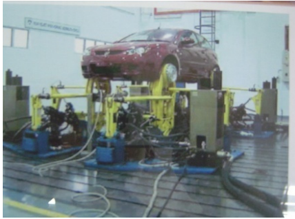
Fig. (7). Multi-axial spindle coupled road simulator.
