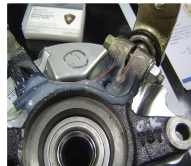
Fig. (6). Strain gauge bonded at critical stress location.
