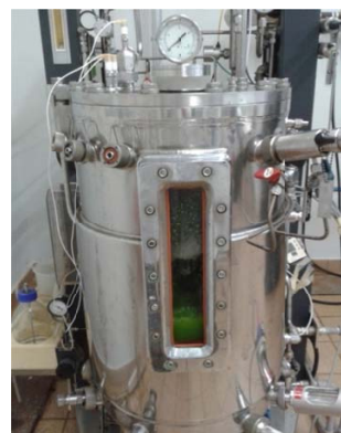
Fig. (6). High quality grade pilot scale fermenter for Chlorella vulgaris heterotrophic cultivation at Campinas State University – Brazil. In partnership with Petrobras (author's personal archive).
