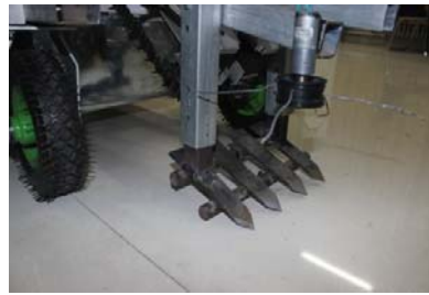
b. Digging shovel
