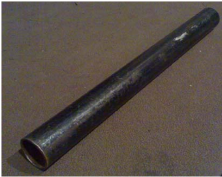
Fig. (11). Metallic tube adopted for the calibration test.
