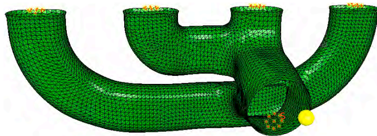
Fig. (23). IBEM model of exhaust manifold with an equivalent point source.
