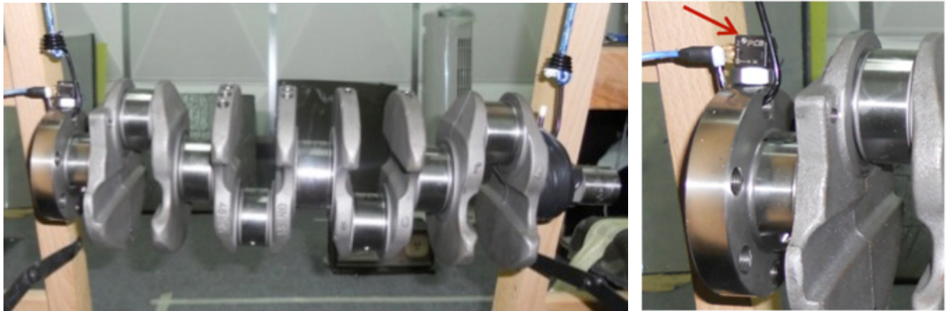
Fig. (10). Crankshaft experimental set-up for modal analysis with highlight of triaxial accelerometer.
