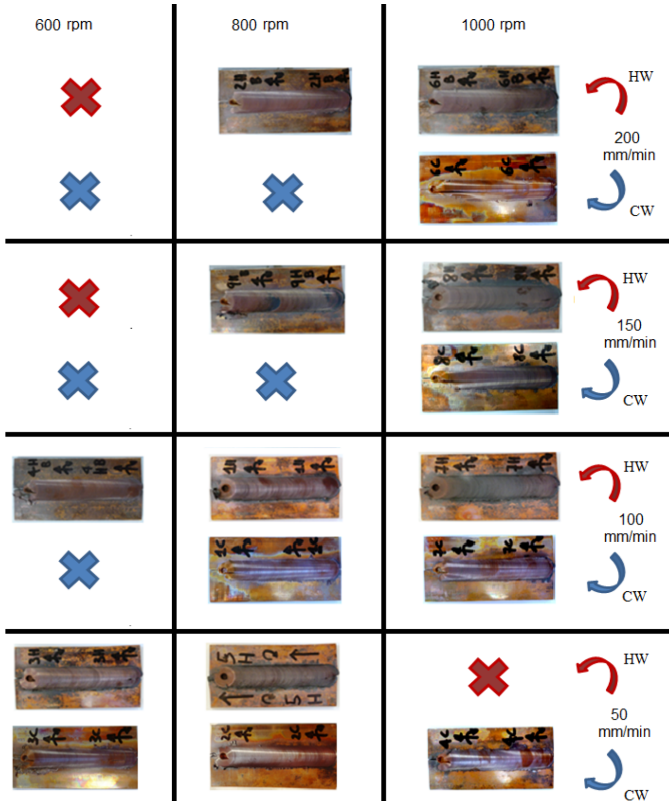
Fig. (3). Hot (HW) and cold (CW) welds. The “x” symbols refer to test cases excluded from the design of experiments.
