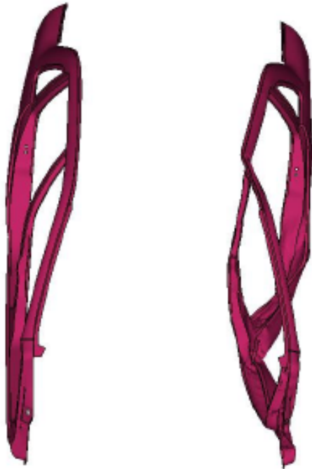
Fig. (9). Side surround deformation.
