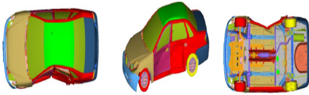
Fig. (13). The crash effect after improvement of B-pillar.
