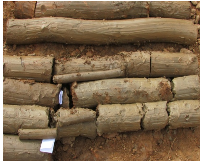
Fig. (9). Weak zone of landslide detected in drilling.
