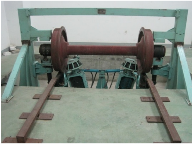
Fig. (16). Wagon wheel set rolling bearing fault diagnosis test bench.
