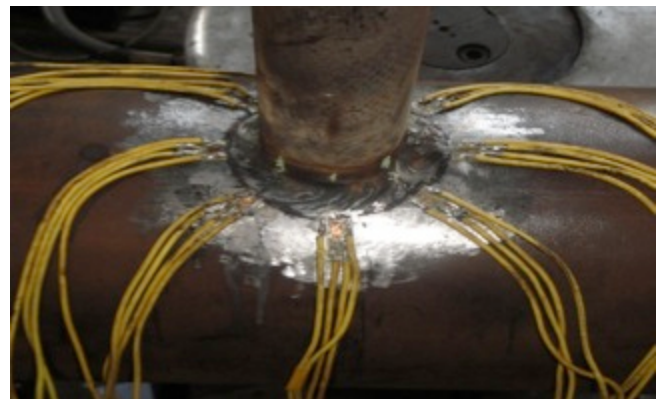
Fig. (4). Arrangement of strain gage.
