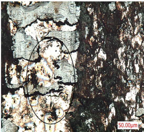
Fig. (5). Wear morphology under dry friction condition and oil lubrication condition ( \times 1000 ).
