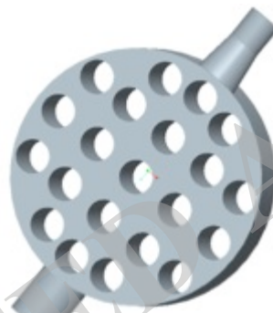
(a) Cylindrical heat exchanger's fluid model
