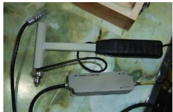
Fig. (5). Modal test system. (a) Test system sketch. (b) Experiment model. (c) Experiment field. (d) Exciting hammer and amplifier.
