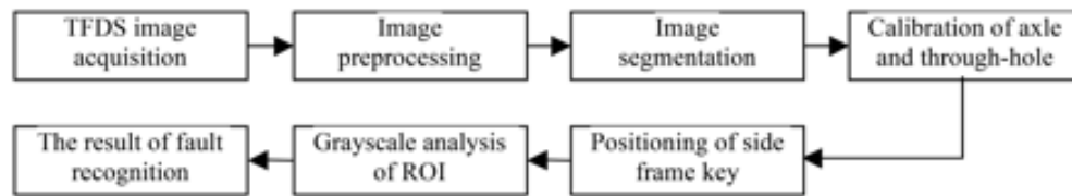
Fig. (1). The automatic fault detection scheme of the side frame key.
