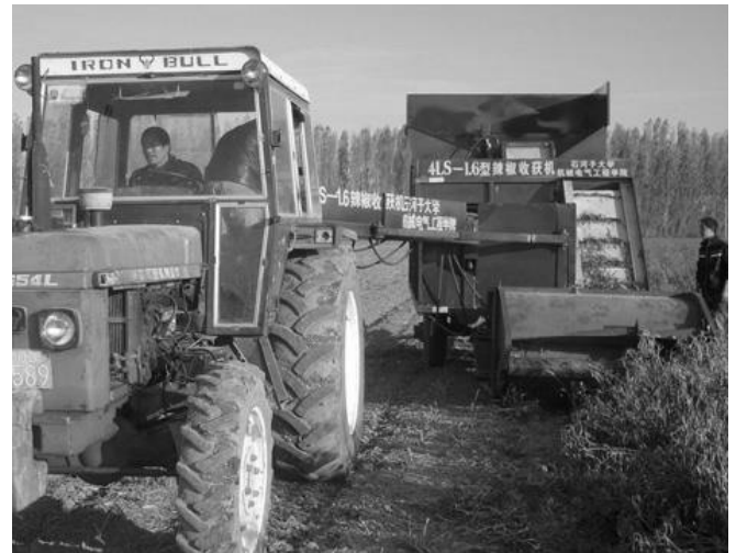
Fig. (11) The photo of the chili pepper harvester's picking test on farm.
