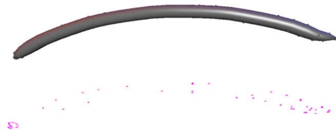
Fig. (5). Deformed model that is predicted by SA scheme. The points set (lower drew in red color) is Key Points selected. The prediction process is only at these points.
