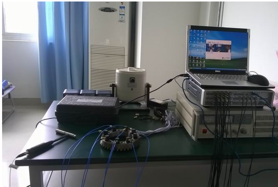
Fig. (10). The layout of experimental modal test.
