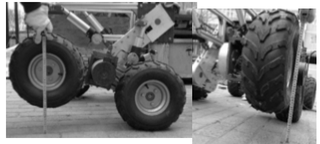
Fig. (6). Motion measurement graphic of the front wheel linear actuator 1.
