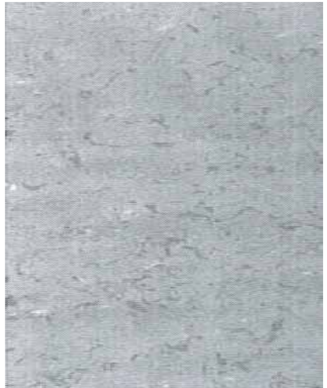
Fig. (8). The structure of the fifth layer shown for sample # 1 (Ni is the main component), x200.
