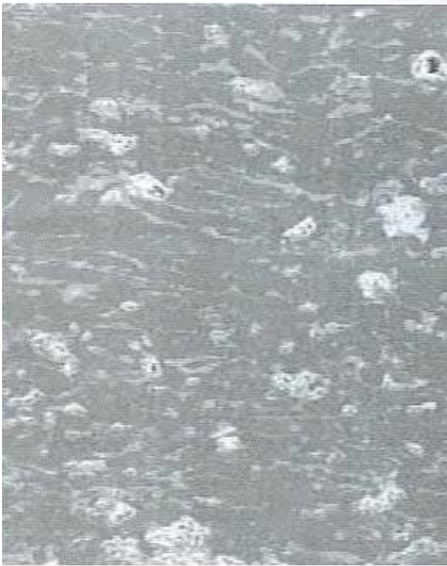
Fig. (5). The structure of the second layer shown for sample # 1 (dark phase: alumina-aluminum oxide, light phase: nickel), x200.
