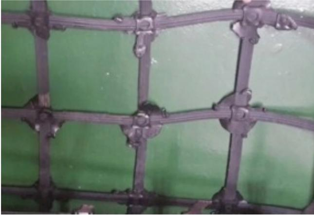
Fig. (1). The steel-plastic geogrid.
