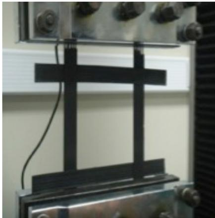
Fig. (3). Universal material testing tensile geogrids.
