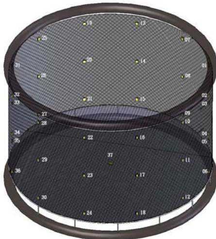
Fig. (3). Placement and numbering of LED markers on the net cage.
