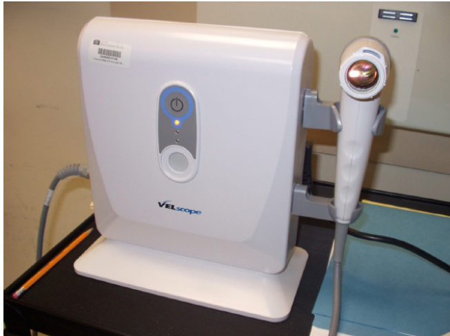
Fig. (3). The VELscope system from LED Dental Inc., White Rock, British Columbia, Canada. It consists of a light source which emits an intense excitation blue light (400-460 nm) and a handpiece with a selective filter for direct visualization.
