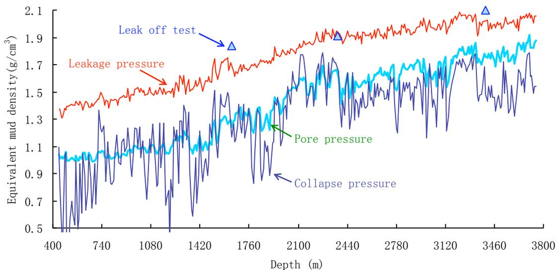
Figure 3 Analysis results of drilling safe density window in some piedmont structure
