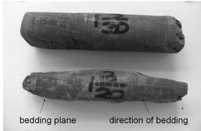
Figure 1 The bedding plane in hard brittle shale of piedmont structures
