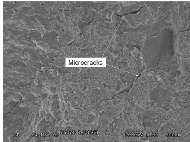
Figure 2 The scanning electron microscope photographs of hard brittle shale of piedmont structures (boost 100 times)
