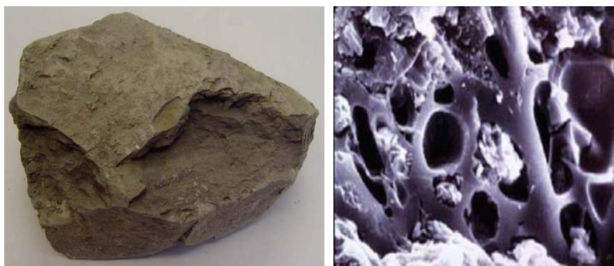
Fig. 4 shale rock and shale gas pores(Steve Drake, 2007)
